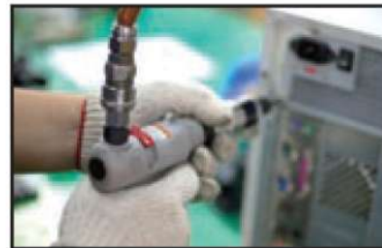
► Operation of Auto Shut-Off Screwdriver
